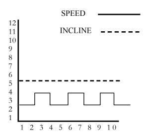
The **Cardio Program** is designed to vary the treadmill Speed, while maintaining a constant Elevation.
